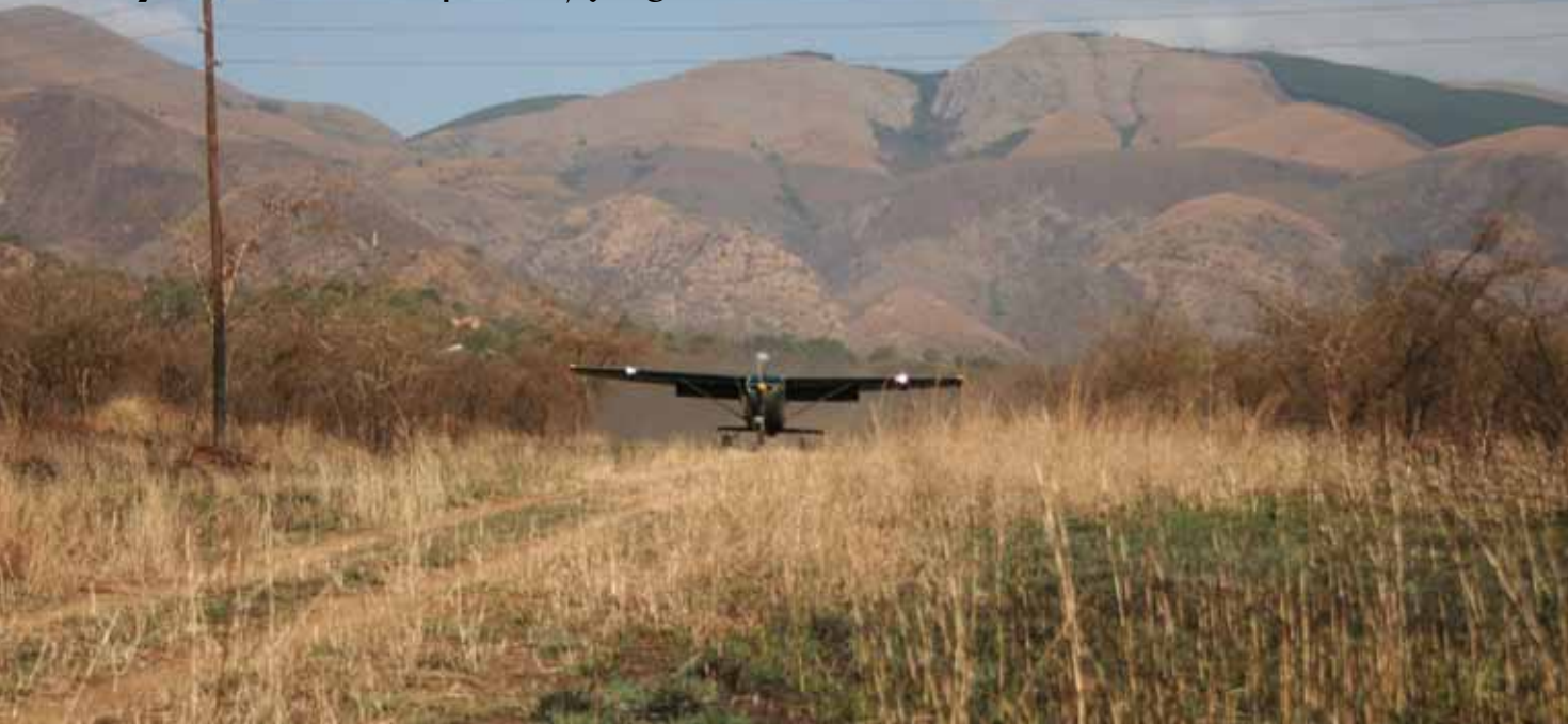
Landing safely under power lines on a narrow bush track, the 172 has full flap and is tail-down for a positive touchdown at lowest possible speed
